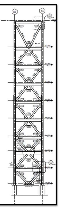
the 9<sup>th</sup> and 10<sup>th</sup> level. The locations of the braced frames help resist lateral loads from all directions. These locations can be found in figure 6 in the foundation section.
